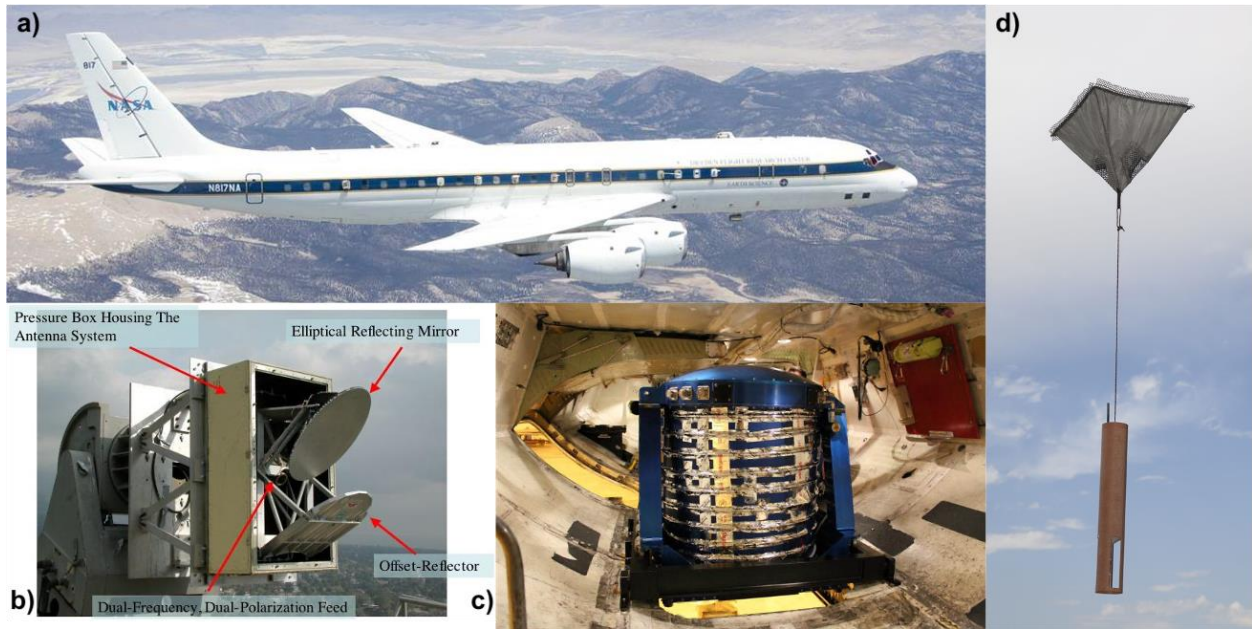
Figure 5: (a) NASA DC-8 aircraft, (b) Third-Generation Airborne Precipitation Radar (APR-3), (c) Doppler Aerosol WiNd Lidar (DAWN), and (d) dropsonde instrumentation used during the CPEX and CPEX-AW field campaigns to sample TOC and their near-storm environments (Images source: NASA).
