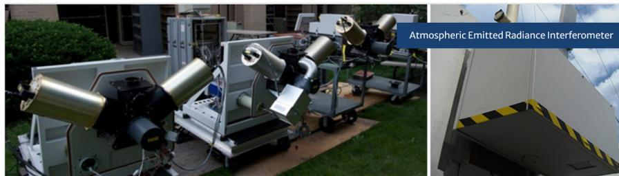
Figure 2.8 The Atmospheric Emitted Radiance Interferometer (AERI) instrument (<https://www.arm.gov/capabilities/instruments/aeri>)
