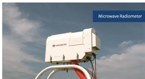
Figure 2.7 Microwave Radiometer (<https://www.arm.gov/capabilities/instruments/mwr>)
