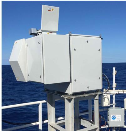
Figure 3.5 The M-AERI instrument deployed on a research vessel during the ACAPEX campaign. (<https://www.flickr.com/photos/armgov/37907508371/in/album-72157647477310974/>)
