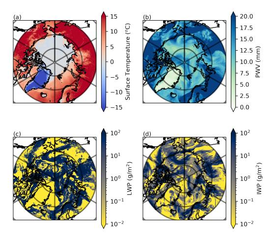
FIGURE 2.1: Four example GFDL fields that go into calculating upwelling radiance using PCRTM: (a) Surface temperature, (b) Precipitable water vapor (PWV), (c) Liquid water path (LWP), (d) Ice water path (IWP). Everything except the northern hemisphere polar region (defined as poleward of 60°N) is masked out.
