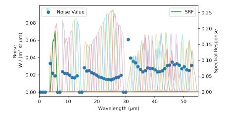
FIGURE B.1: Expected values of each channel's noise plotted against the channel's center wavelength (blue scatter) for the TIRS instrument. Masked channels due to instrument limitations are listed with noise values of 0. The spectral response function (SRF) for each channel is shown with a colored line.
